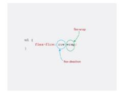
flex-flow broken down in bits
